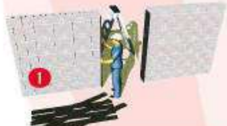
1 Vertical frame work erected, end secured and horizontal level taken
