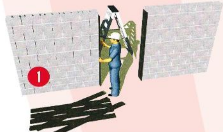
1 Vertical frame work erected, end secured and horizontal level taken
