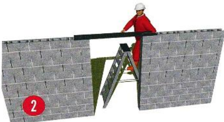
2 Lintel is placed in position
